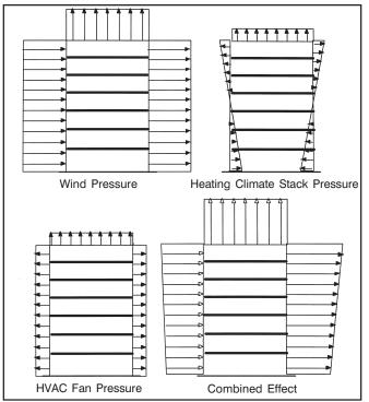
Figure 3: Combined wind, stack and fan pressure.
